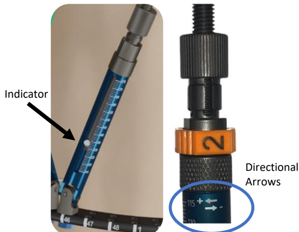
Figure 10: Indicator reflects strut length; adjust per prescription
